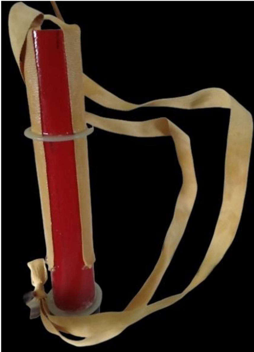
Figure: The first motor mount tube assembly by UREPL (with epoxied kevlar thread)
