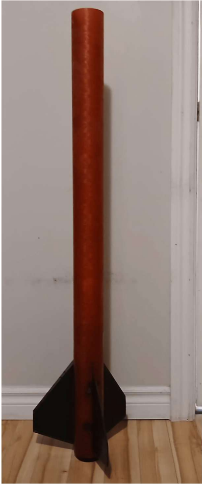
Figure: Fins attached with the Fin Alignment Jig
